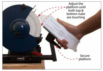
Loosen the platform locking knob and adjust the platform so that both the top and bottom nubs are touching the grinding wheel keeping the RESTING EDGE flat against the platform as shown above. Once you are at the correct setting, secure the platform by tightening the platform locking knob.
