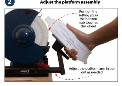
Loosen the red lever so you can adjust the position of the platform arm in or out. Place the setting jig on the platform so the preferred RESTING EDGE is flat against the platform. Adjust the platform arm in or out until the bottom nub of the setting jig touches the grinding wheel leaving at least a 1/4" to 3/8" gap between the platform and the grinding wheel as shown above. Tighten the red lever to lock the platfrom arm in place.
